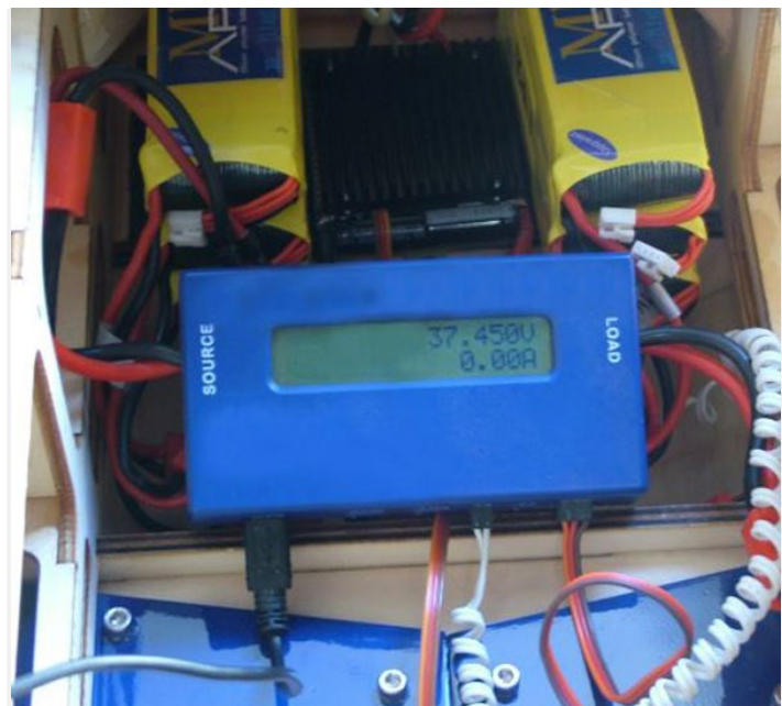
A power meter is a handy piece of equipment to have to check how your airplane power system is operating.
